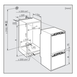
Before installing the appliance make sure the housing unit is the correct size. Specified ventilation gaps must be maintained in order to ensure the appliance functions correctly.
